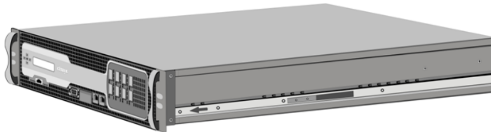
Figure 3-1. Attaching inner rails
